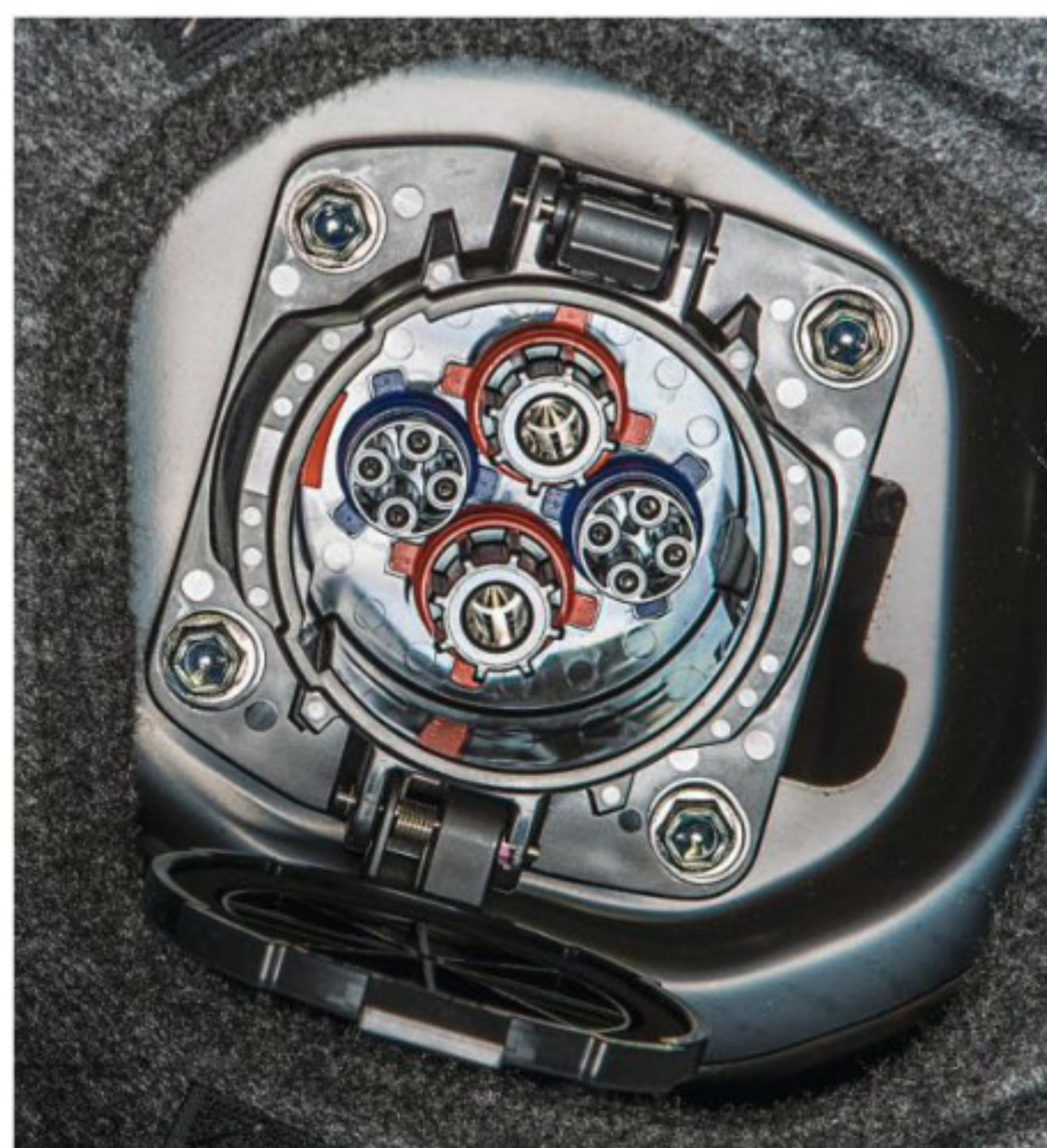
Clockwise from above: Not an engine but a power-control unit to manage the fuel cells and the system's batteries; the Mirai hits streets this fall; this plug allows the car to serve as a backup-power source for your house in case of electrical blackouts.
