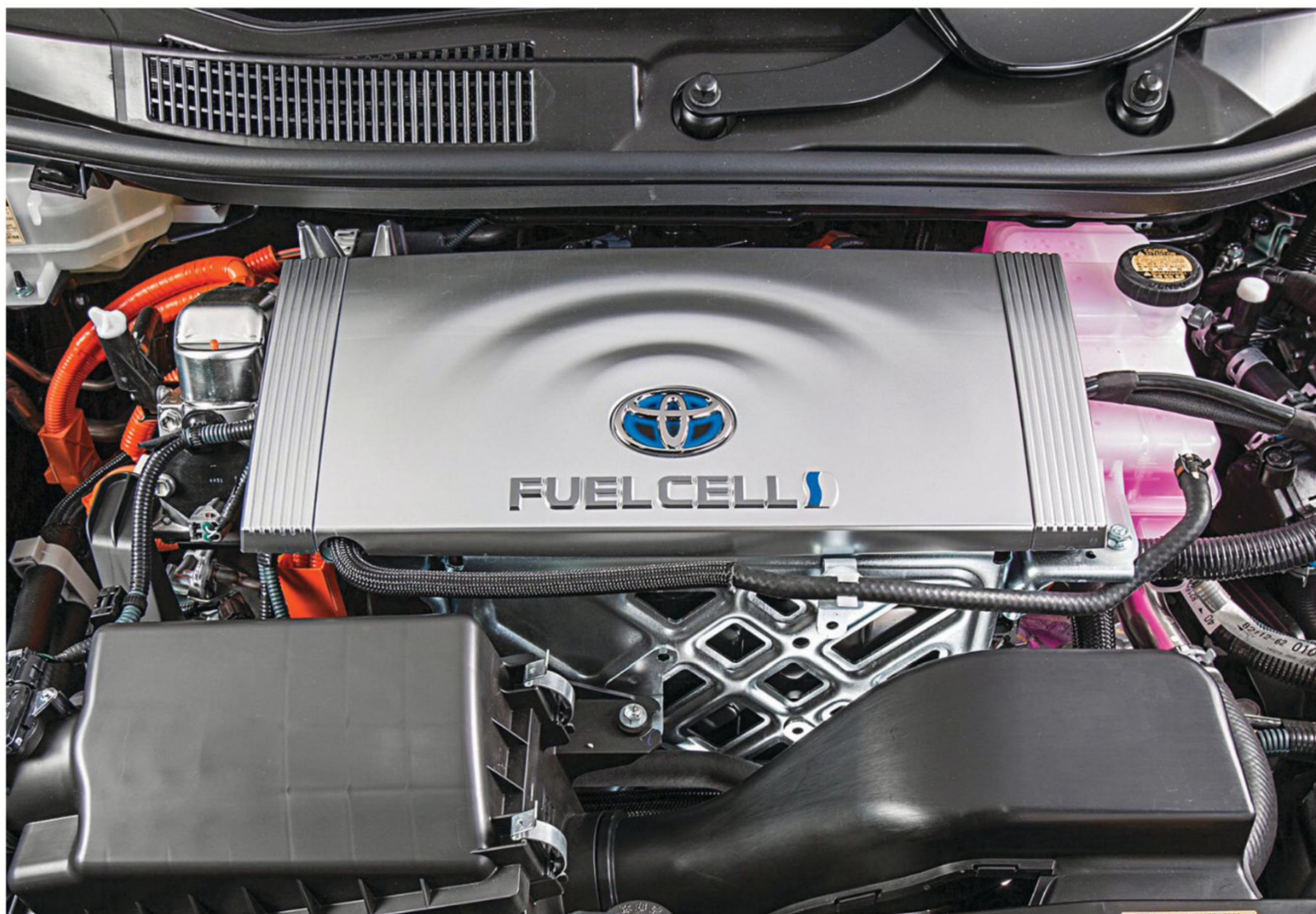
Clockwise from above: Not an engine but a power-control unit to manage the fuel cells and the system's batteries; the Mirai hits streets this fall; this plug allows the car to serve as a backup-power source for your house in case of electrical blackouts.
